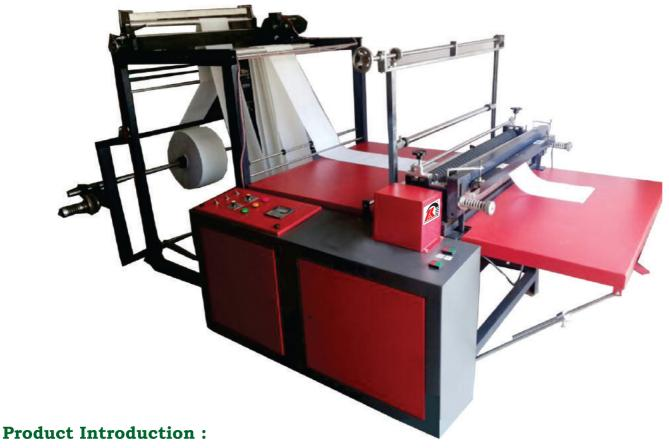
This Machine is Automatic Non woven Roll to Sheet cutting machine, it is use full to cut different size of Non woven fabric sheet to make non woven bags, Pillow covers,Bad sheet and it can also cut different size of Wax strip.
